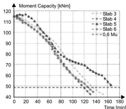
**Fig. 7. Comparison of variation of moment capacity with fire exposure time in different slabs**
