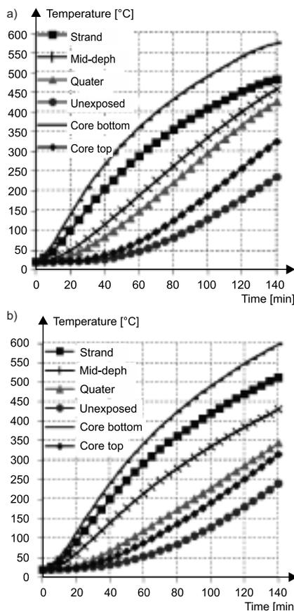
**Fig. 5. Comparison of measured and predicted sectional temperatures in siliceous and carbonate aggregate concrete slabs: a) siliceous aggregate concrete slab; b) carbonate aggregate concrete slab**
