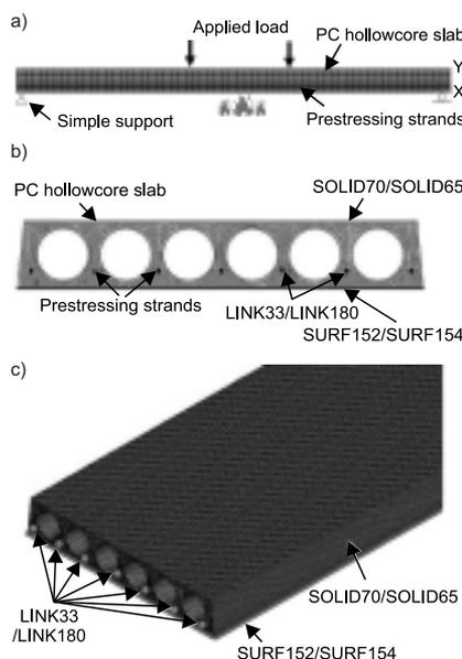
Fig. 4. Layout of a typical PC hollowcore slab and its discretization for fire resistance analysis: a) typical hollowcore slab exposed to fire; b) discretization of cross-sectional of hollowcore slab; c) discretized hollowcore slab in longitudinal direction
