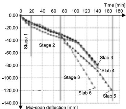
**Fig. 6. Comparison of measured and predicted mid-span deflections in different slabs**
