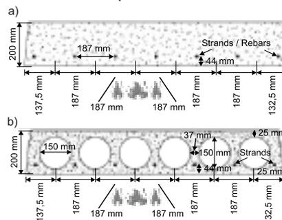
**Fig. 1. Comparison of cross-sectional profiles of typical fire-exposed prestressed concrete: a) solid slab; b) hollowcore slab**
