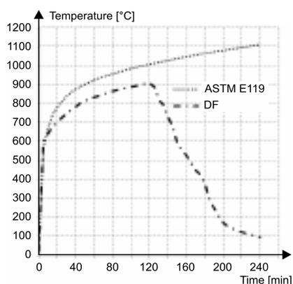
Fig. 3. Time-temperature curves of fire exposure
