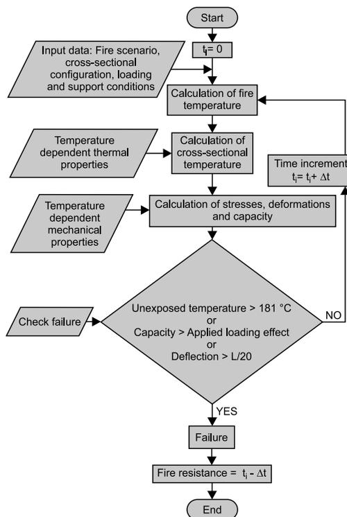
Fig. 2. Flowchart showing steps associated with fire resistance analysis of hollowcore slabs
