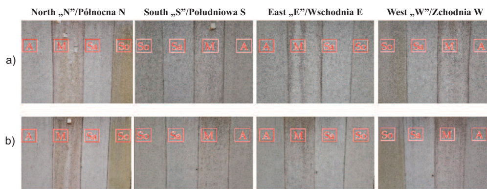
Test stations with thin-layer plaster samples oriented according to the cardinal directions for the following textures: a) lambskin; b) bark beetle
