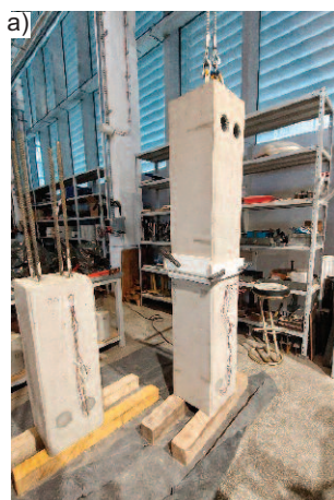
Photo 1. The process of preparing the test specimens: a) traditional joint with dowels – element before pouring the upper channels; b) bolted system joint – view of the bolted elements
