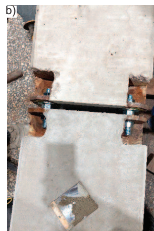
Photo 1. The process of preparing the test specimens: a) traditional joint with dowels – element before pouring the upper channels; b) bolted system joint – view of the bolted elements
