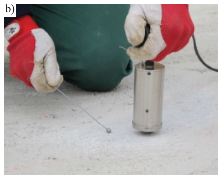
Photo 3. Measurements using: a) the Impulse-Response method; b) the Impact-Echo method
