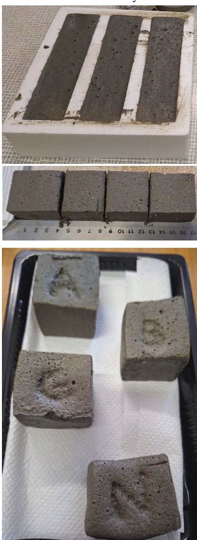
Photo 1. Geopolymer mortar before exposure, 2 weeks after preparation
