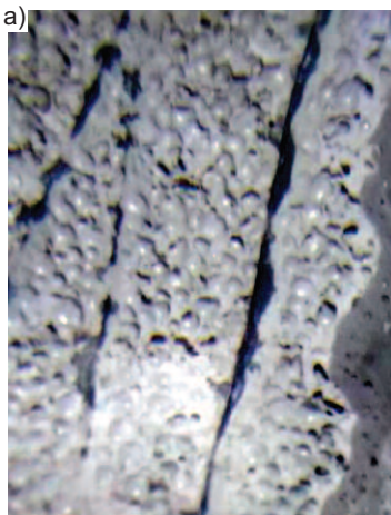
Photo 5. Destroyed organic coating: a) partially melted HDG coating; b) field microscope photos – magnification: 50x [26]
