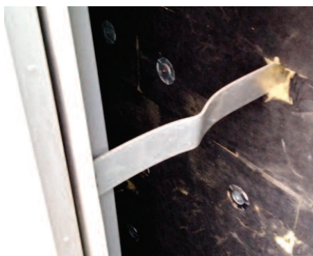
Photo 1. Aluminum bracket with mounting deformations
