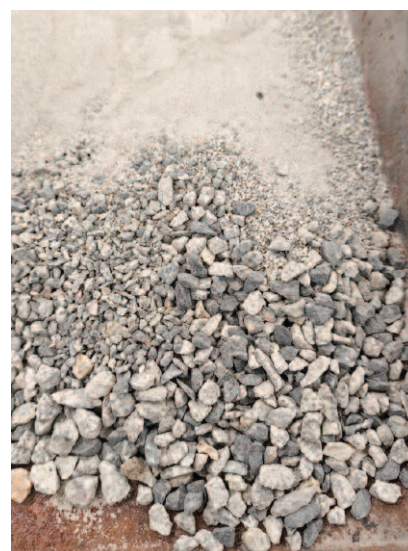
Photo 2. Granite aggregate 0/31.5 after sieve analysis
