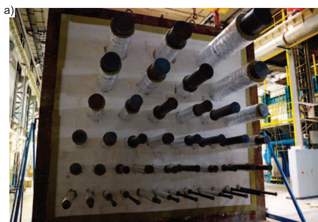
The test specimen before fire resistance testing: a) unheated surface; b) heated surface
