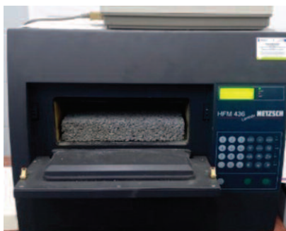
Photo 2. Thermal conductivity test using the NETZSCH HFM 436 apparatus
