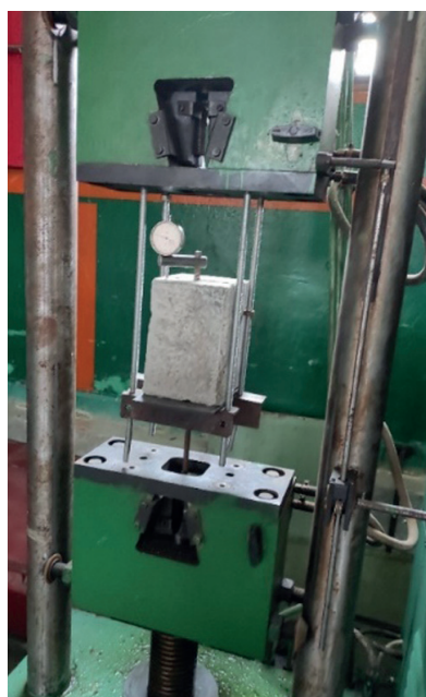
Photo 4. Testing of a sprayed concrete sample
