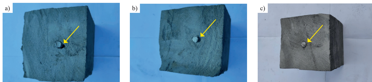
Photo 5. Cross-section of damaged specimens made according to the shotcrete application scheme: a) scheme I (up to 5°); b) scheme II (5°–10°); c) scheme III (10°–15°)
