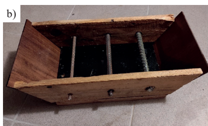
Photo 2. Mould for the preparation of: a) test cubes, sprayed concrete cubes; b) reinforced cuboid samples
