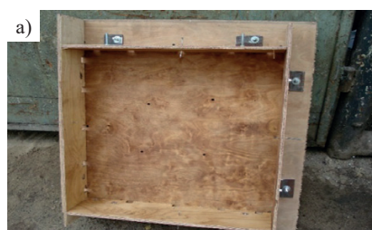
Photo 2. Mould for the preparation of: a) test cubes, sprayed concrete cubes; b) reinforced cuboid samples
