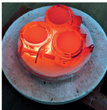
Photo 2. Heated molds inside a Hot Pot
