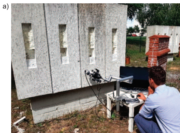
Photo 1. Test stand on the campus of the Bydgoszcz University of Technology during tests with the Keyence Series VHX-7000 microscope (a) field, (b) laboratory
