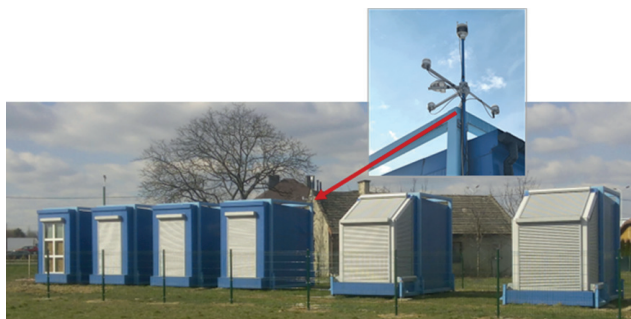
A weather station located on one of the helioenergetic chambers
