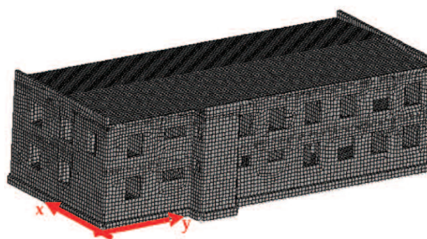
Fig. 1. Three-dimensional model of the analysed building with a finite element mesh
