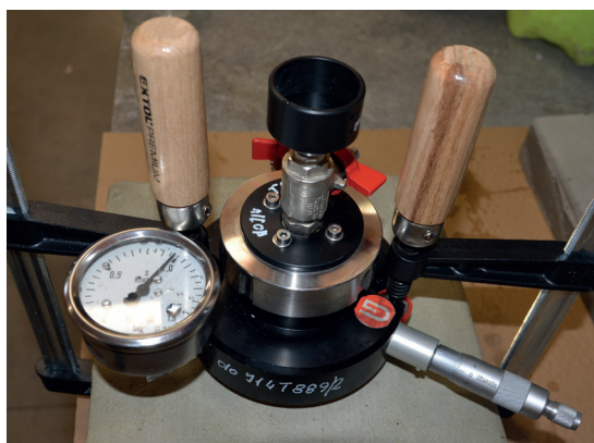
Photo 5. GWT equipment during mortar sample testing Fot. 5. Aparatura GWT w trakcie badania próbki zaprawy
