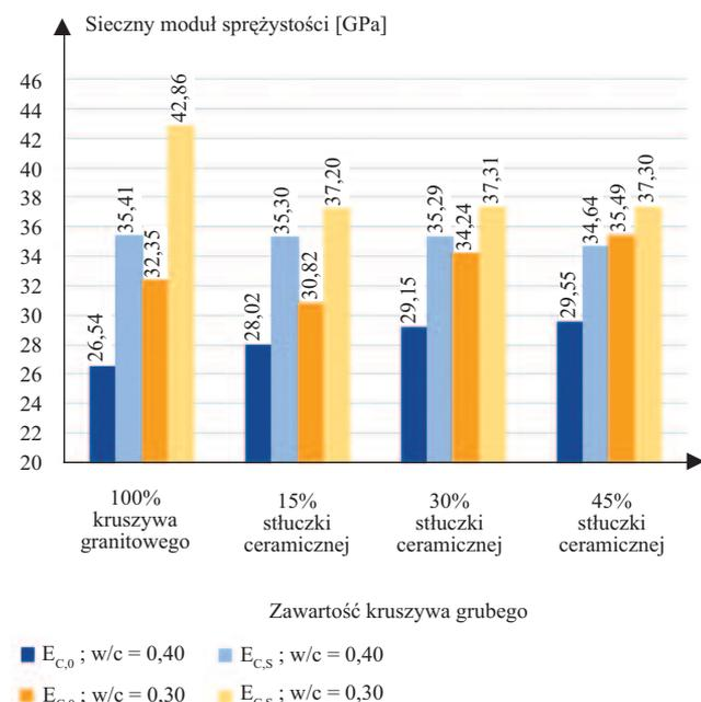
**Fig. 3. The test results for the secant modulus of elasticity**
