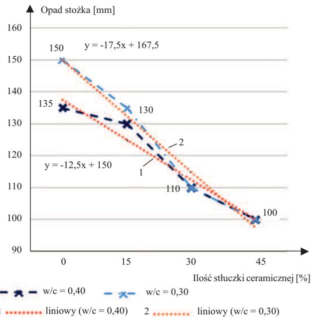
Fig. 2. The results of testing the consistency of the concrete mixture using the cone fall method
