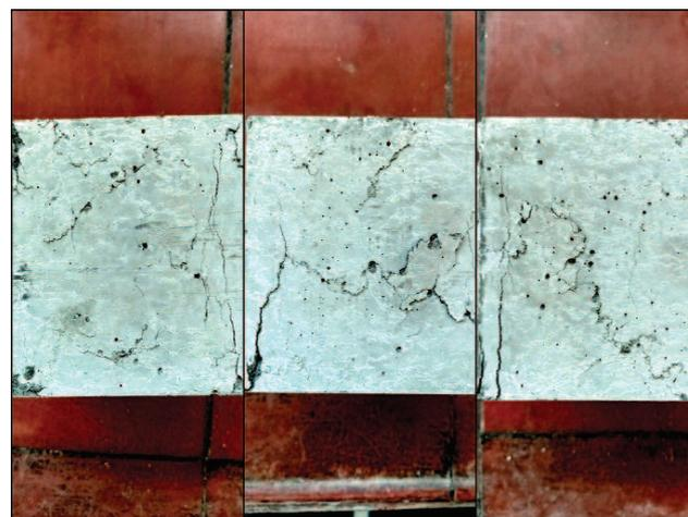
**Photo 2. The course of cracks in B0 samples subjected to compressive strength testing. Failure pattern typical of high-strength concrete**
