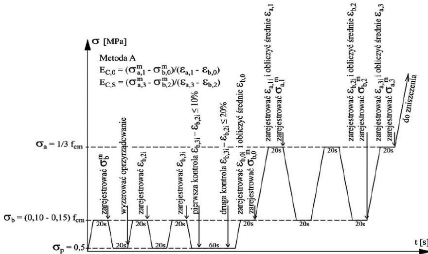
Fig. 1. Load diagram in method A for determining the initial and stabilized secant modulus of elasticity [27]
