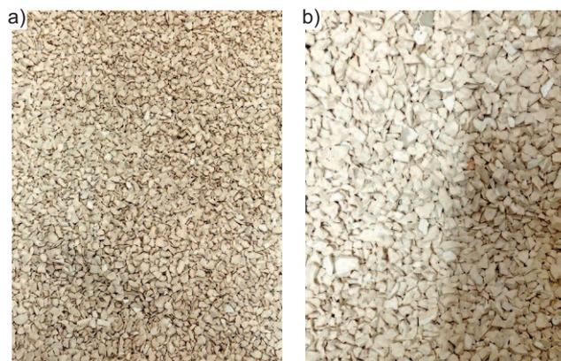
**Photo 1. Ceramic recycled aggregate used in the research; fraction: a) 4 – 8 mm; b) 8 – 16 mm**
