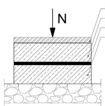
**Fig. 1. Principle of the compression resistance test: 1 – concrete slab 20 x 20 cm, 4 cm thick; 2 – tested bitumen-polymer coating; 3 – metal pressure plate**
