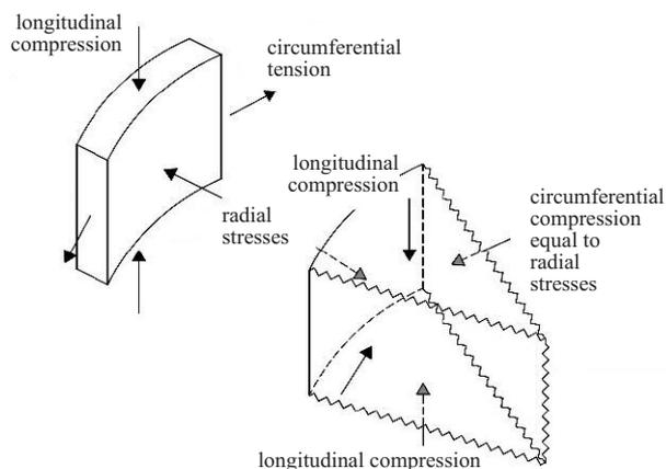
**Fig. 1. State of stresses in a CFT column**
