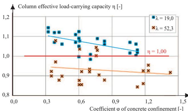
**Fig. 3. Relationship between the effective load capacity  $\eta$  of CFST columns and their slenderness  $\lambda$  and the coefficient  $\phi$  of concrete confinement (which is a measure of the circumferential stiffness of the steel tube) for 48 experimentally tested columns**
