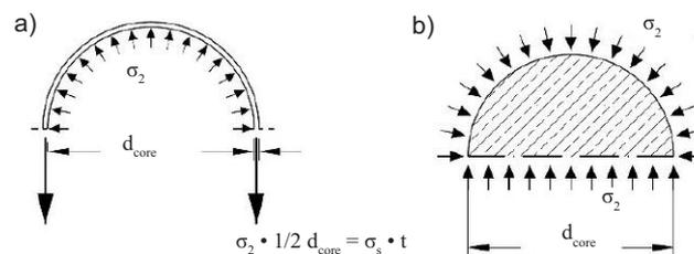
**Fig. 2. Stress equilibrium in the cross-section of the CFST column: a) steel tube; b) concrete core**
