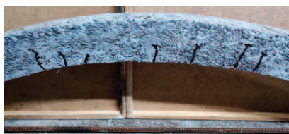
The arch with contours of cracks after the test
