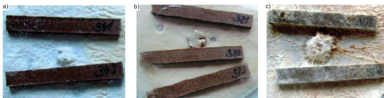
**Photo 1. Samples of composite reinforced with oat husks after exposure to: a) *Coriolus versicolor*; b) *Gloeophyllum trabeum*; c) *Coniophora puteana***
