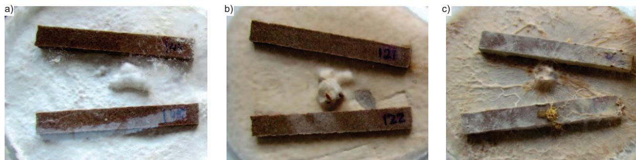
**Photo 3. Samples of composite reinforced with rice husks after exposure to: a) *Coriolus versicolor*; b) *Gloeophyllum trabeum*; c) *Coniophora puteana***
