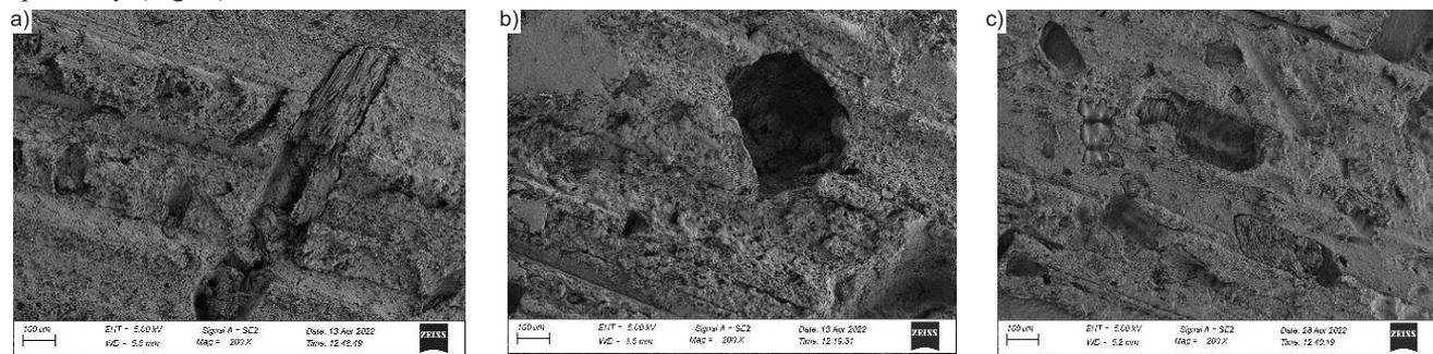
**Photo 4. Microstructure of the husk-reinforced composite's surface: a) oat; b) millet; c) rice following the exposure to *Coniophora puteana*, 200x magnification**
