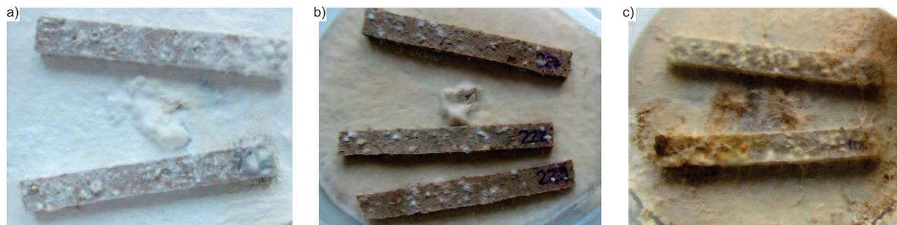
**Photo 2. Samples of composite reinforced with millet husks after exposure to: a) *Coriolus versicolor*; b) *Gloeophyllum trabeum*; c) *Coniophora puteana***
