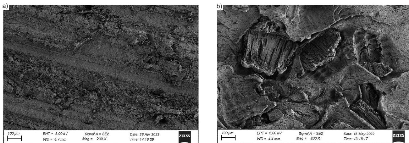
**Photo 3. Surface microstructure of NFPC composites with PVC matrix reinforced with pulverised oat husks: a) before ageing; b) after ageing**
