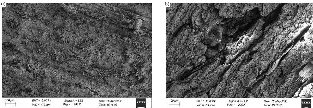
**Fig. 4. Surface microstructure of NFPC composites with PVC matrix reinforced with pulverised millet husks: a) before ageing; b) after ageing**
