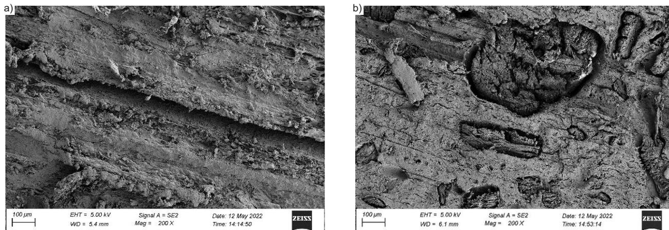
**Photo 2. Surface microstructure of NFPC composites with PVC matrix reinforced with pulverised rice husks: a) before ageing; b) after ageing**
