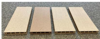
**Photo 1. Chamber profiles with the addition of pulverized rice, oat and millet husks**
