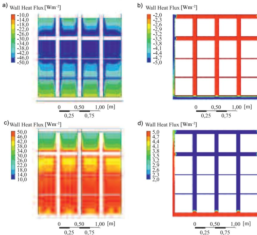
Fig. 8. Density of heat flux for glass and window frame in contact with air: a) and b) external; c), and d) internal (Type 2)
