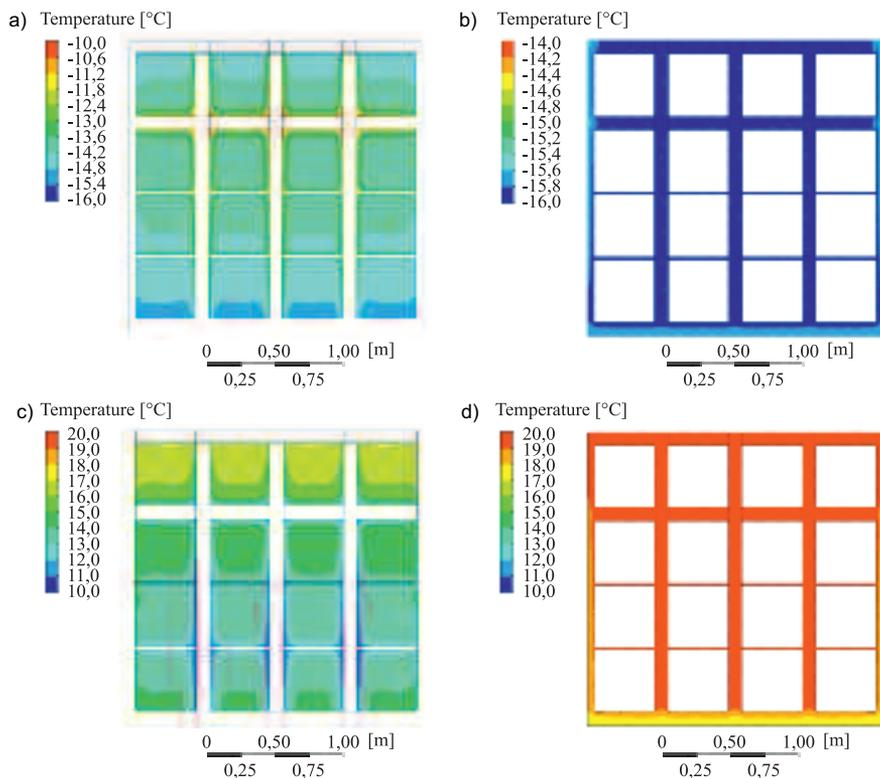
**Fig. 5. Temperature distribution field for glass and for window frame in contact with air: a) and b) external; c) and d) internal (Type 1)**
