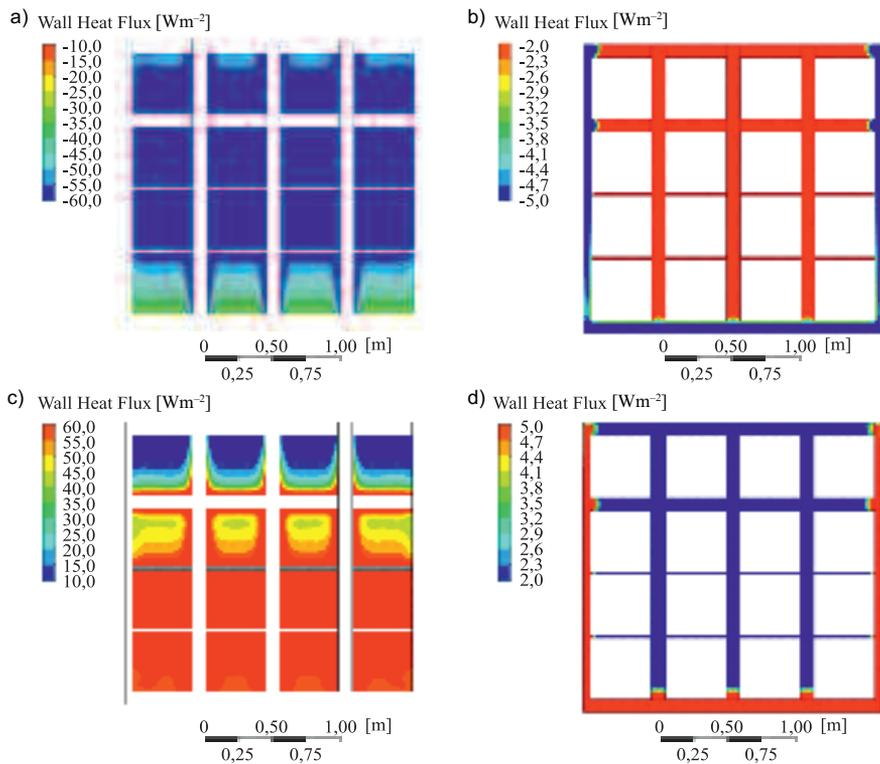
**Fig. 6. Density of heat flux for glass and for window frame in contact with air: a) and b) external; c) and d) internal (Type 1)**
