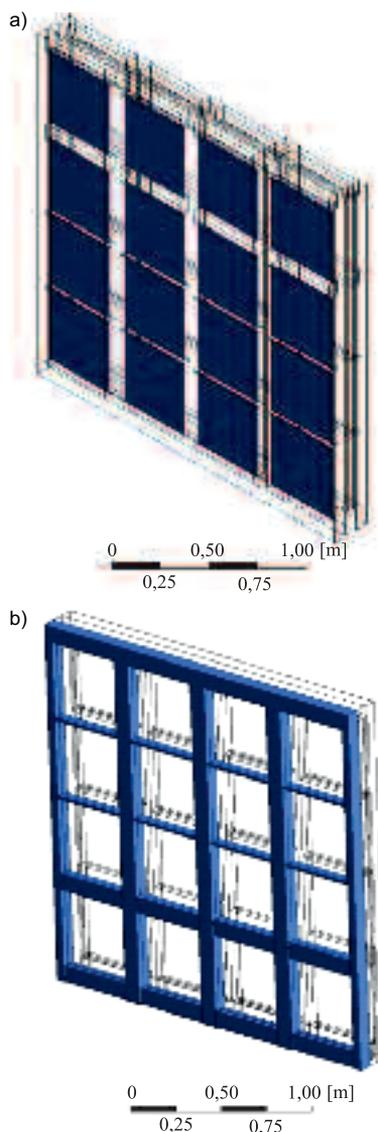
**Fig. 2. Numerical model of window joinery: a – glass, b – frame**
