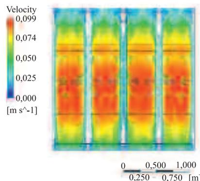
**Fig. 4. Distribution of air flow velocity in the air gap in the window**
