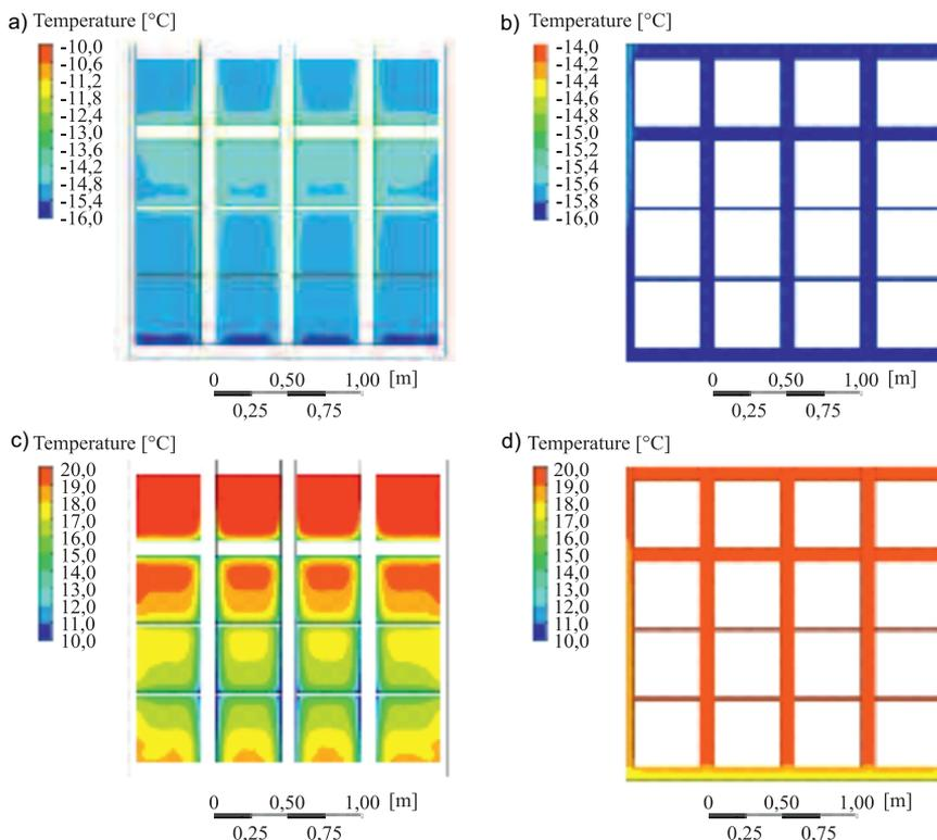
Fig. 7. Temperature distribution field for glass and for window frame in contact with air: a) and b) external; c) and d) internal (Type 2)
