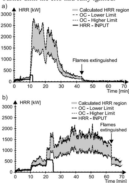
Fig. 4. Heat input and output from burner and wooden crib (note that ignition of the crib occurred after 10 minutes, so the propane was switched off after 11 minutes; a) – PIR panels; b) – stone wool panels
