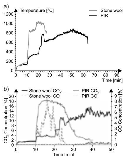
Fig. 5. Weighted average temperature of upper layer – burner and wood crib experiments (a); CO and CO<sub>2</sub> concentration at doorway – burner and wooden crib experiments (b)
