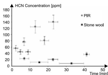
Fig. 3. HCN concentrations – propane burner experiments (the horizontal bars indicate duration of bubbler sampling)
