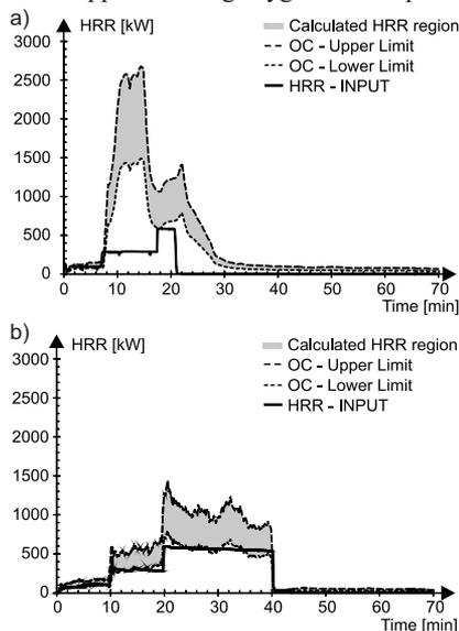
**Fig. 1. Heat input and output from tests with burner only. OC refers to measurements based on oxygen consumption calorimetry: a) – PIR panels; b) – stone wool panels**
