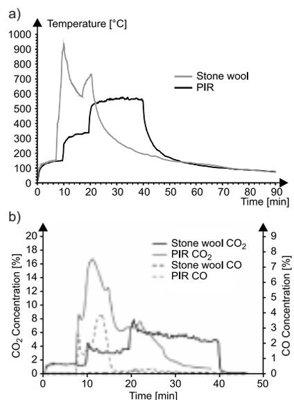
**Fig. 2. Volume-weighted average temperature of upper layer – burner only experiments (a); CO<sub>2</sub> and CO concentrations at doorway – burner only experiments (b)**
