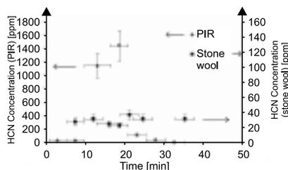
**Fig. 6. HCN concentrations – propane burner and wooden crib experiments (horizontal bars indicate duration of bubbler sampling)**
