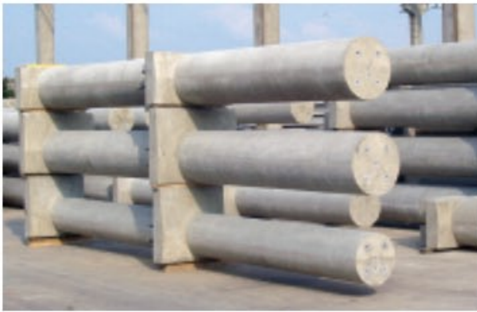
Fig. 4. Two-storey-high circular columns in self-compacting, high-strength concrete
