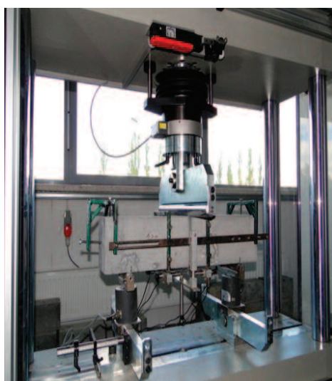
Photo 1. The stand for testing residual bending tensile strength
