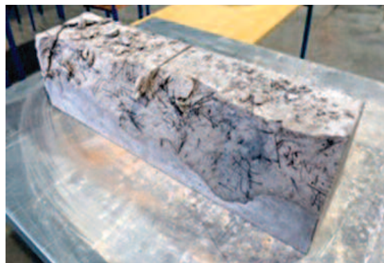
Photo 3. The sample image of beam specimen after heating at a temperature of 800°C
